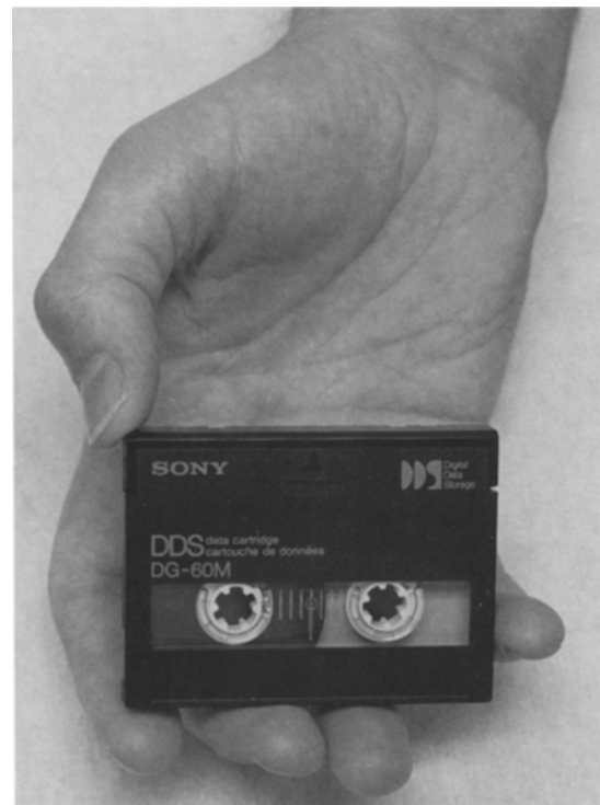
Fig 5. 4-mm digital audio tape (DAT) used for image backup and archiving.
