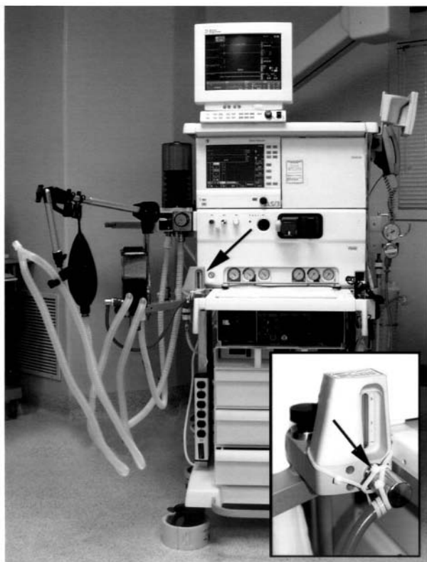
FIGURE Depicts the securance of the fresh gas flow hose to the fresh gas outlet of the Datex gas machine to prevent the erroneous connection that was present in this obstetrical case.
