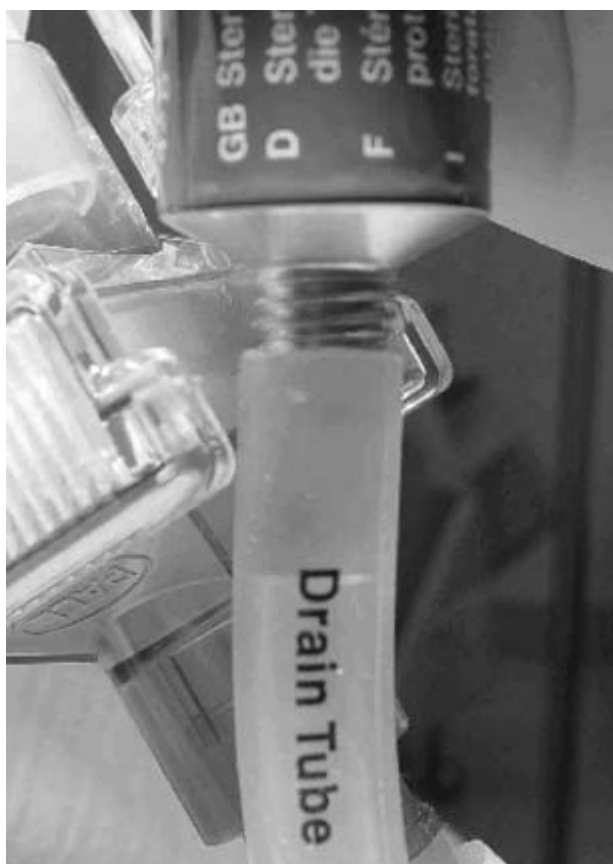
FIGURE Injection of a column of lubricant into the drain tube by pressing the tube flush against the opening of the drain tube.
