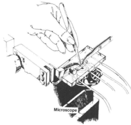
FIGURE 4 Study of chemically skinned muscle cells. Each cell is mounted horizontally between two clamps in a bathing chamber filled with a calcium free relaxing solution.
