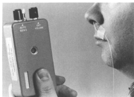
FIGURE 2 View of the monitor and the placement of the sensor.
