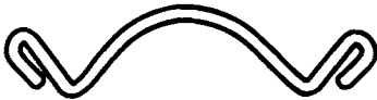
Part no. 1 Scale: 1:1 (can be used as a template) Material: Stainless steel spring wire
