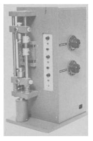
the downward movement. The second microswitch cuts off the power to the heating element. Heater temperature and solenoid 'pull' are variable, and the positions of the chucks, the element and the microswitches are adjustable.
