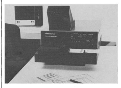
The Corning semi-automation fluorometer/densitometer will scan any flat clear electrophoresis media and allows quantitation of isoenzyme electrophoresis tests by colourimetric and fluorometric methods. Simple quantitations can be done in 12·5 s and results are presented as tracings on data cards. The instrument includes a microprocessor to control
