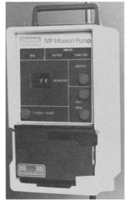
intravenous container is empty. Weighing 5 kg, the pump is supplied with an integral pole clamp, is mains powered and can also be operated from an external 12 V supply.
