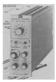
output of 5V d.c. The instrument responds equally well to input signals of amplitudes from 10 mV r.m.s. to 500 V r.m.s. and has an input impedance of 100 k $\Omega$ . The convertor can be used with unipolar signals and also has calibrated zero suppression with a resolution of 0·1% permitting suppression of the static portion of a complex signal. Any waveform can be accepted.
