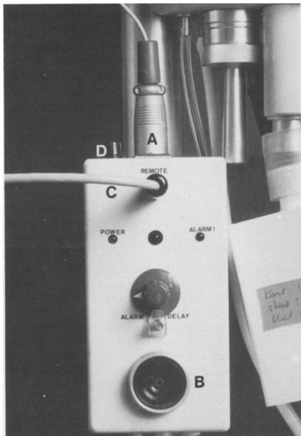
Fig. 2. The box "processing" the information from the photocell: A – cabel from the photocell, B – sound emitting unit, C – cabel to the control switch, D – "off" and "on" dial
