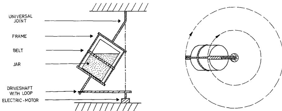
Fig. 1: Culture apparatus. Left: side view. Right: viewed from above
