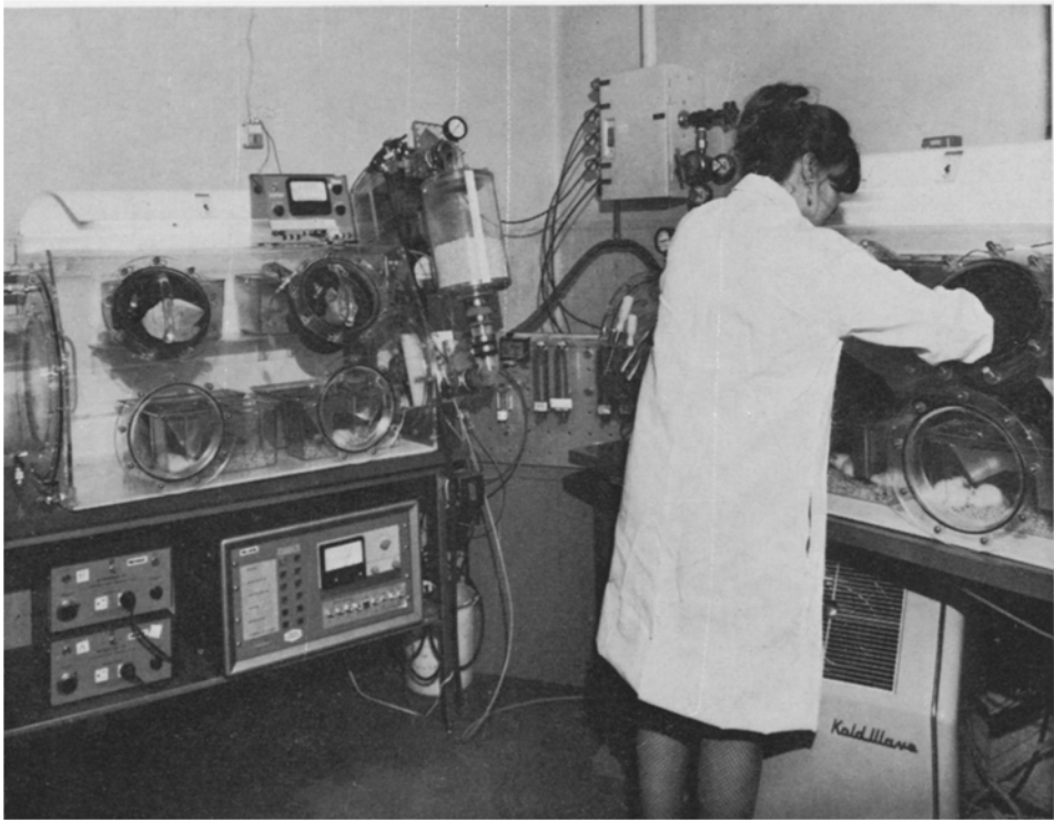
Fig. 1. Closed environmental system (CES-4). A dual chamber system for the chronic exposure of animals to potential spacecraft cabin atmospheres. Chamber A (helium-oxygen) is shown on left, chamber B (nitrogen-oxygen) at right. Master control unit for both chambers is shown beneath chamber A.
