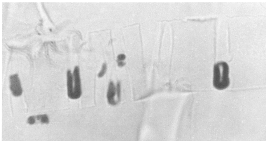
Fig. 1. Light microscopic photograph of a Nuclepore polycarbonate filter with ob/ob mouse erythrocytes in the pores. Note profiles indicative of erythrocyte folding. 2,000 \times
