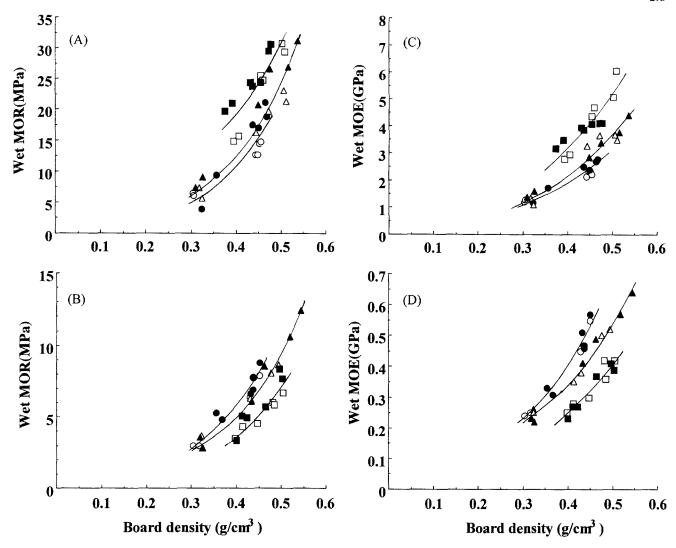
Fig. 2. Wet bending properties of sandwich panels. Wet MOR in parallel (**A**) and perpendicular (**B**) directions and wet MOE in parallel (**C**) and perpendicular (**D**) directions. Veneer thicknesses of sandwich pan-
