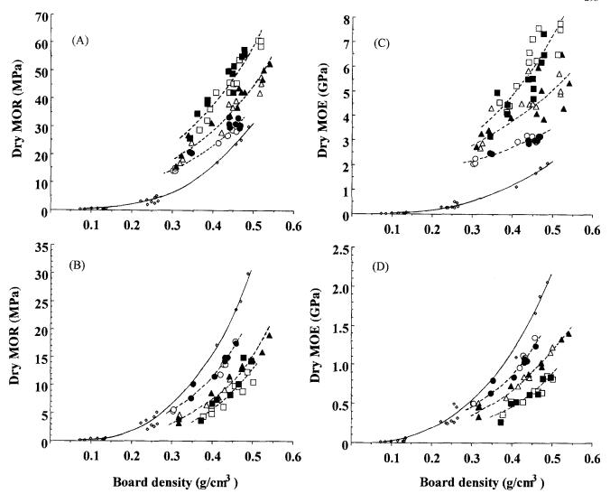
**Fig. 1.** Dry bending properties of sandwich panels and low-density fiberboards. Dry MOR in parallel (**A**) and perpendicular (**B**) directions and dry MOE in parallel (**C**) and perpendicular (**D**) directions. Veneer thickness of sandwich panels are 0.55 mm (*circles*), 1.0 mm (*triangles*),
