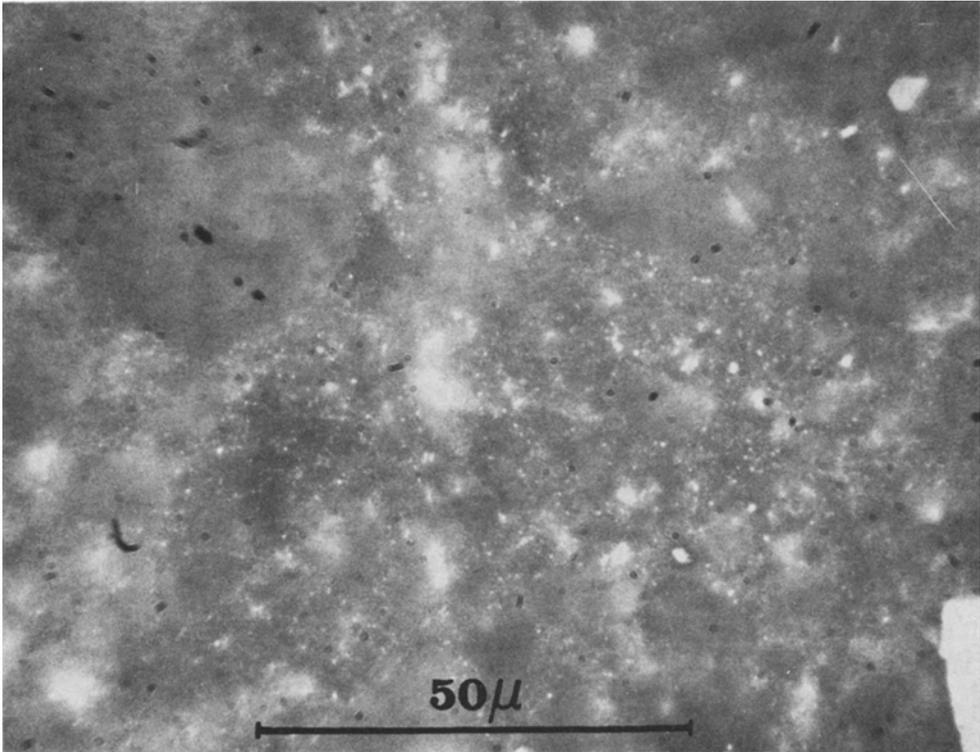
Fig. 2. High-magnification image of a portion of a BCBx clast in thin section 72275,12, showing disseminated metallic iron grains (white). In addition to relatively large ( $1-2 \mu$ ) grains, a cloud of very tiny ( $\sim 0.1 \mu$ ) iron particles are scattered through the breccia matrix. Reflected light illumination, an oil immersion objective, and high-contrast film were used.
