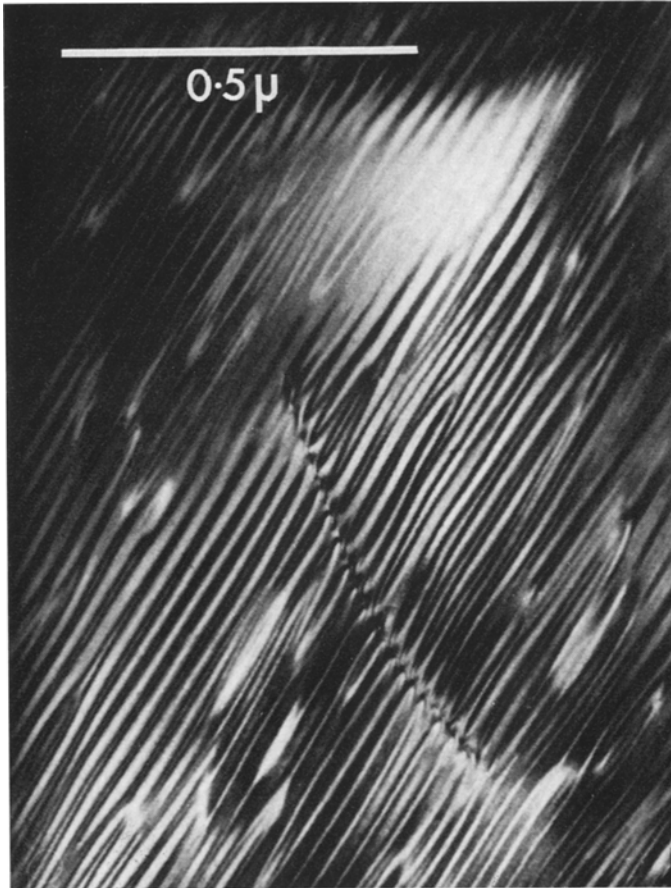
Fig. 2. Electron micrograph of an Apollo 12 pyroxene crystal showing a lamellar development of alternating Ca-rich and Ca-poor regions. (Champness and Lorimer, 1972).
