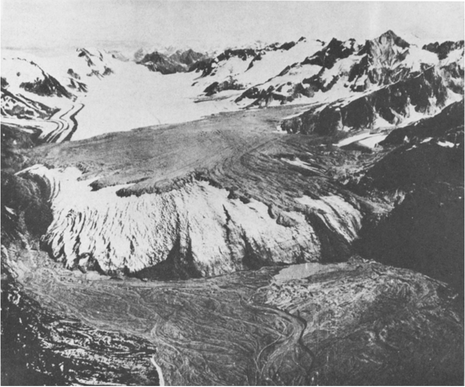
Fig. 8a. Sherman landslide, Alaska. a. Viewed from west. Debris fell from peak at right, and crossed the 2.5 km wide Sherman Glacier. Thickness of debris 3–6 m; volume 3 \times 10^7 M^3 .
