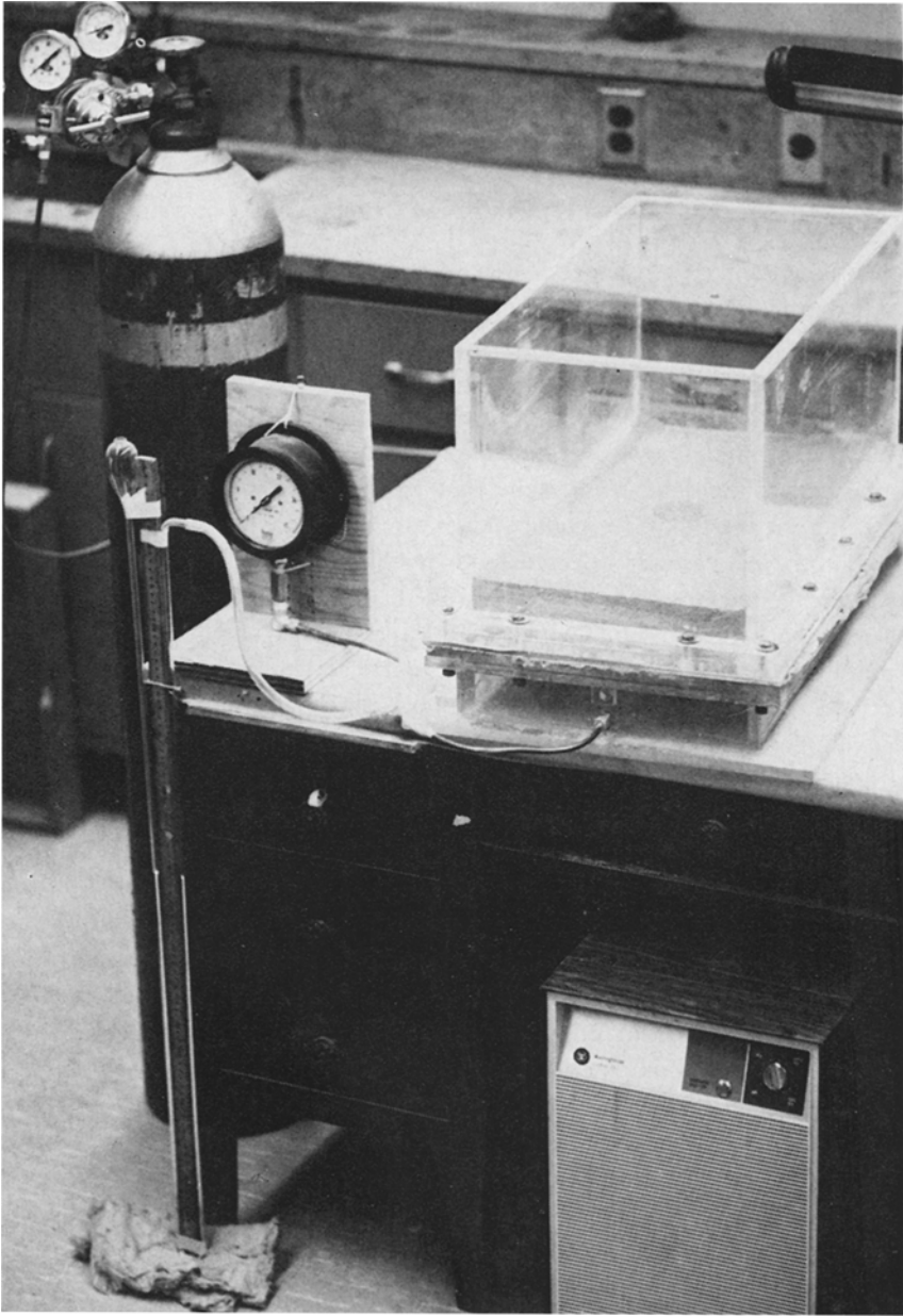
Plate 1. Equipment set-up, showing fluidization chamber, gas pressure and humidity control systems.
