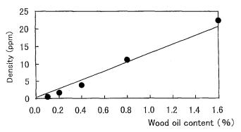
Fig. 8. Calibration curve for the density variation of  $\alpha$ -pinene by gas chromatography corresponding to the concentration of wood oil contained in respective test samples of *C. obtusa*
