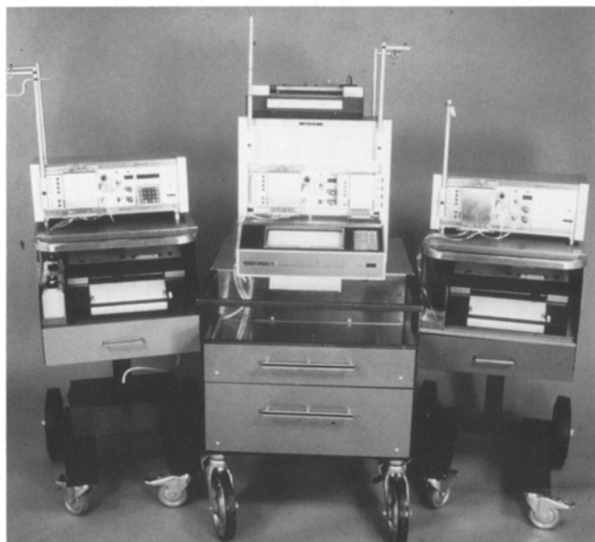
Fig. 4. Our artificial endocrine pancreas (Ulm-Elkhart Version) and two simplified versions as glucose controller and glucose monitor
