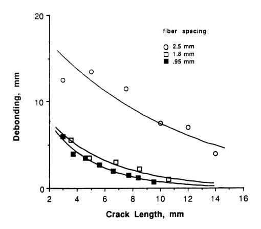
Figure 9. Extent of fiber debonding for three fiber spacings.
