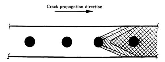
Figure 8. A schematic of fracture surfaces. The different shades indicate consecutive positions of the crack front.
