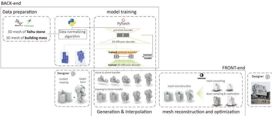
Fig. 4. 3D form finding workflow based on diffusion probabilistic models
