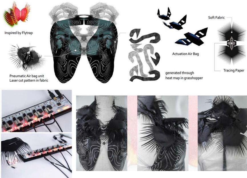
**Fig. 7.** Various prototypes of pneumatic air-bags' structures inspired by muscles and flytrap
