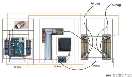
**Fig. 6.** An example of pocket-sized pneumatic system with one portable air pump, one pair of two-sets miniature electromagnetic valves that can control two sets of airbags, and an Arduino toolkit which can connect sensors easily
