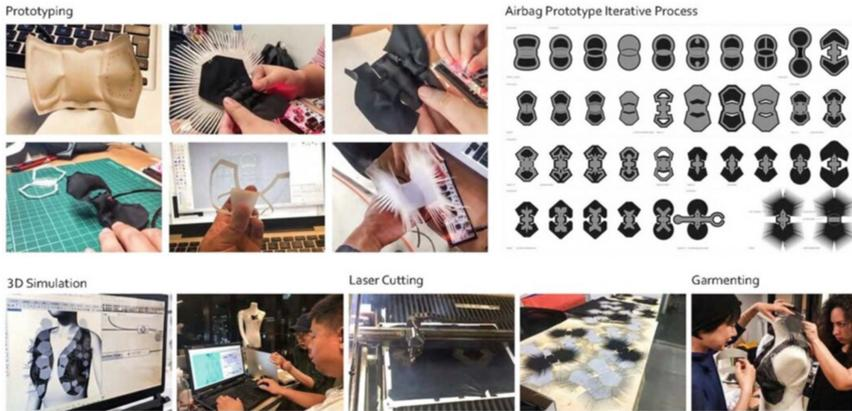
**Fig. 3.** Programable Soft Materials: TPU and silicone and the process of their computed structures supported by Rhino and CAD. The Fig. 3 shows the process of TPU computed structures which was supported by Tongji University College of Architecture and Urban Planning and developed in DigitalFUTURES Shanghai 2018 Workshop
