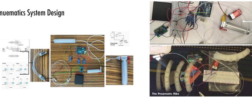
**Fig. 5.** Pneumatic system design. The pictures on the left show how the pneumatic system is designed. The two pictures on the right show the testing of pneumatic system
