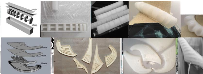
**Fig. 4.** Programable Soft Materials: TPU and silicone and the process of their computed structures supported by Rhino and CAD. The Fig. 3 shows the process of TPU computed structures which was supported by Tongji University College of Architecture and Urban Planning and developed in DigitalFUTURES Shanghai 2018 Workshop
