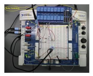
**Fig. 6.10** NI ELVIS II+ board with relay switches
