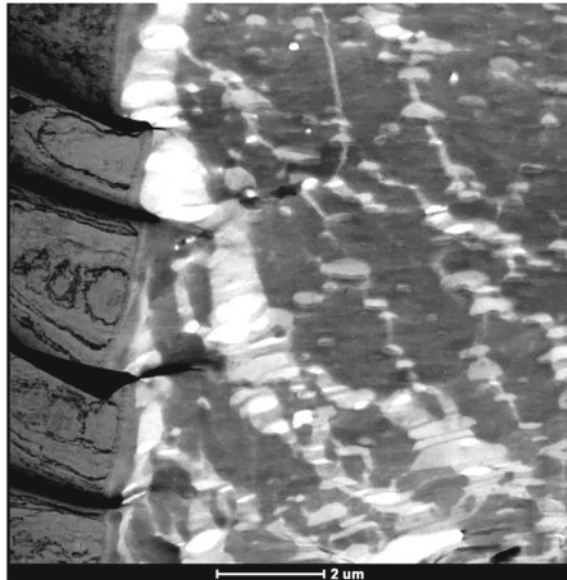
Fig. 64 Video showing the failure behavior of the PPS/Al direct joint in STEM bright-field (BF) mode
