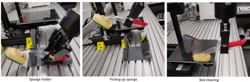
Fig. 10 Automated printer bed cleaning process
