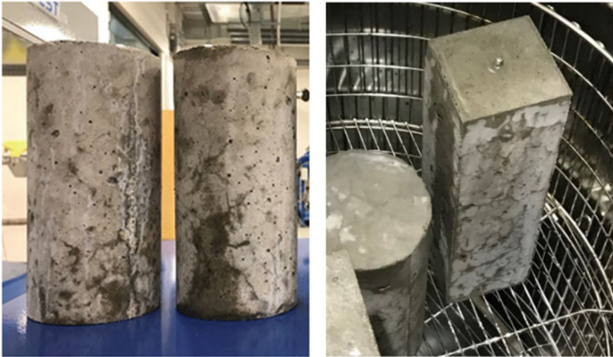
Fig. 3 External map cracking on cylinders and prisms after three cycles of steam curing in an autoclave
