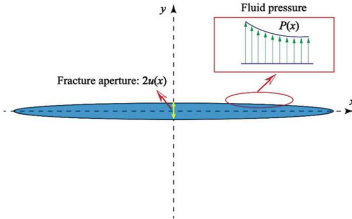
**Fig. 2.1** Fracture pressurized by internal fluid
