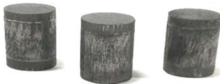
Fig. 4. Coated particle dispersion fuel pellets
