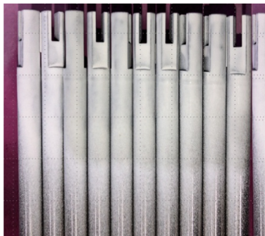
Fig. 11. Weld penetration result
