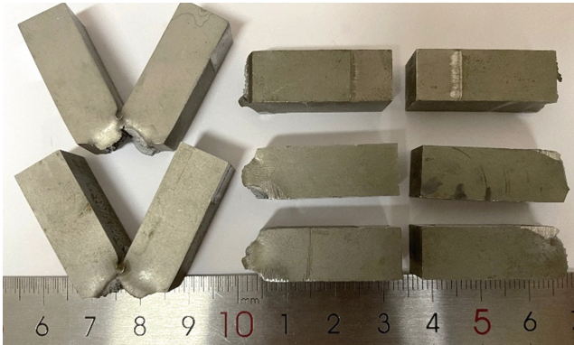
Fig. 3. The impact fracture.
