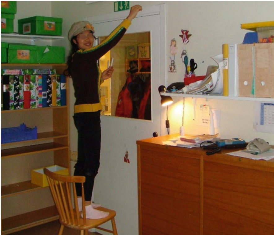
Fig. 9.1 Sampling of settled dust from a door frame in a day care center for analysis of fungal DNA
