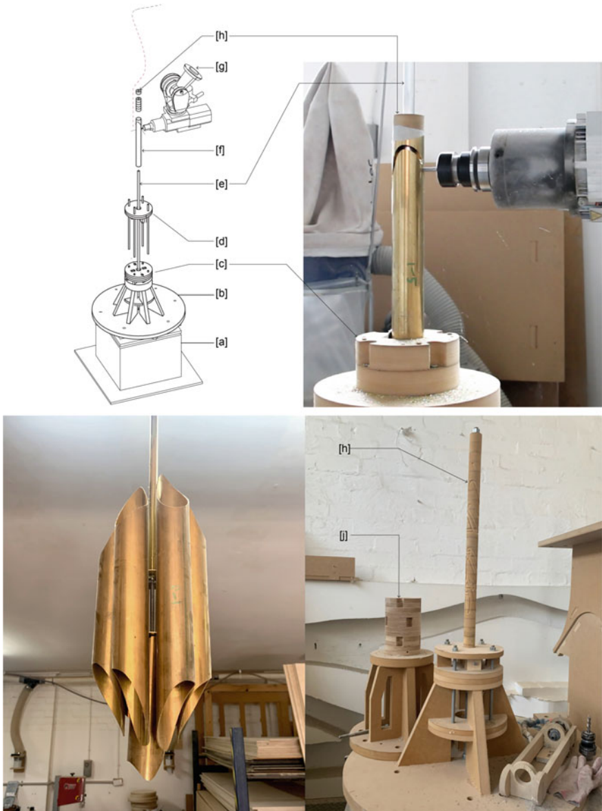
Fig. 2. Top left: Design of the fixture holding the metal tube. Top right: Milling of the brass tube using the fixture. Bottom left: 8-tubes chandelier prototype. Bottom right: Robot fixtures indicating the solid MDF block [h] infill to the brass tube and early fixture prototype [j].
