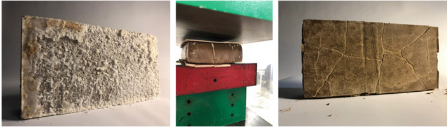
Fig. 4. Salt brick, compression test & resultant brick.
