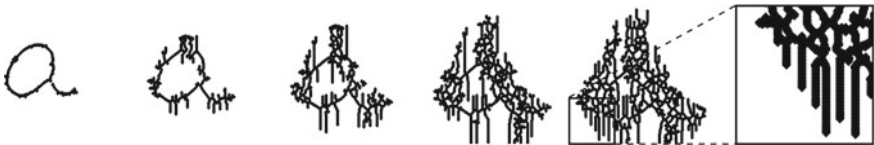
Fig. 5. Square brush redrawn the path as a saw-shaped figure, further guiding the skeleton to grow in other directions.
