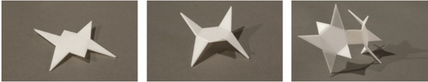
Fig. 3. First 3D printed structures: flat, bent, and a different typology showing the connection.
