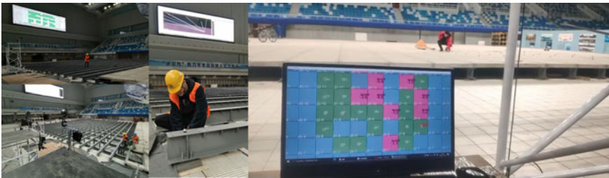
Fig. 8. On-site placement of the motion capture system and the collected point cloud for each marker
