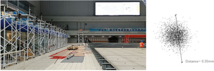
Fig. 7. On-site placement of the motion capture system and the collected point cloud for each marker
