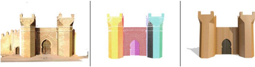
Fig. 6. Three stages of Chellah's gate reconstruction.
