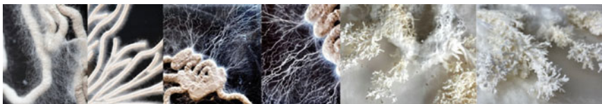
Fig. 6. Clay infused with mycelia robotic extrusions. Overtime, the mycelium began to grow from the organic mixture and wandered around the surface area in search for additional nutrients.
