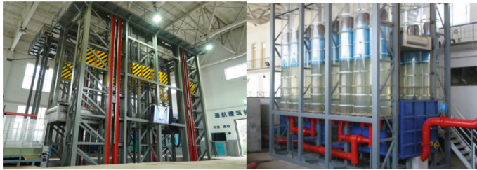
a) Rack and pinion ship lift (3000t)
