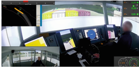
Fig. 2. Main full mission bridge simulator with 360° view at FH.
