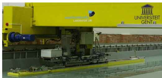
Fig. 4. Towing tank tests: ECMT class Vb.
