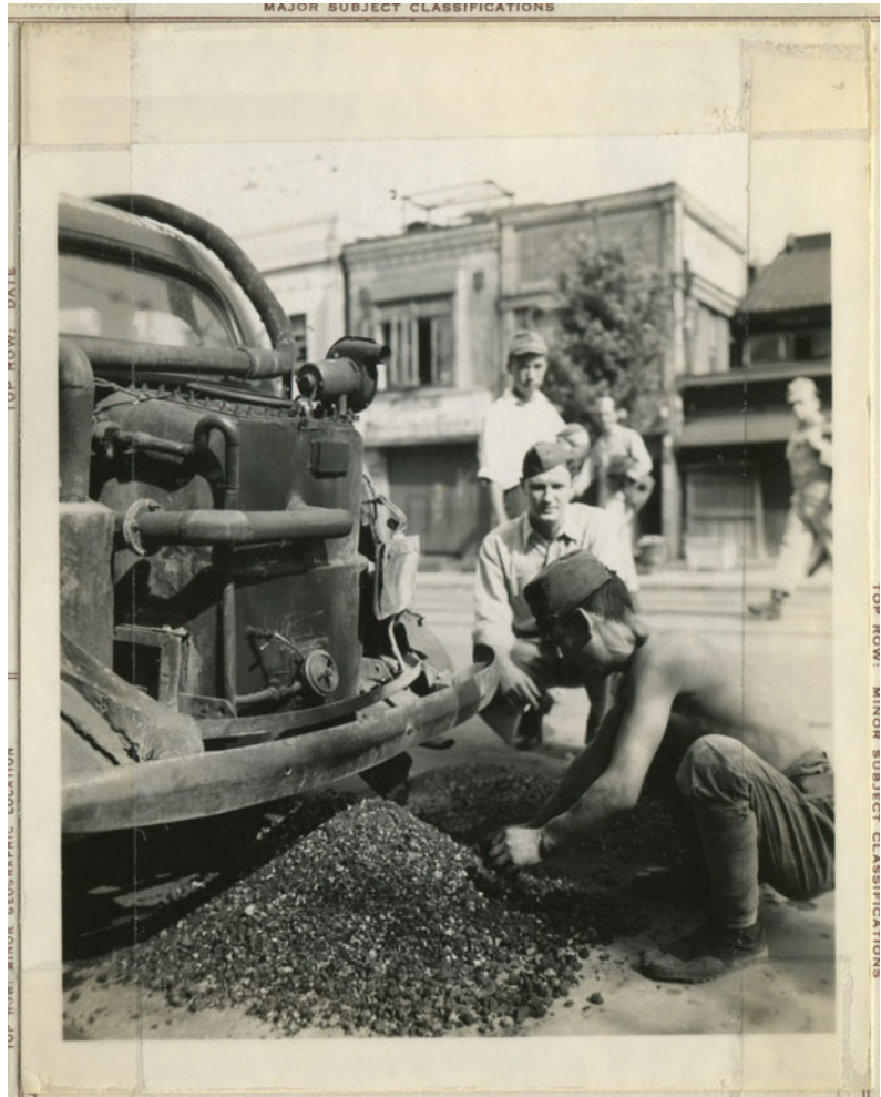
Fig. 4.19 Cleaning up the coal cinders that power this car. Tokyo or Yokohama. US Marine Corps (USMC) photo. 127-135403. NARA. Coal-powered vehicles can frequently be found in photographs taken by the occupying forces
