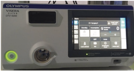
Fig. 9 Video system center unit with both image processor and light source
