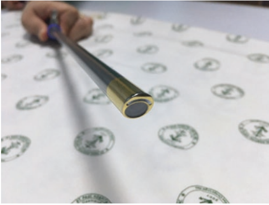
Fig. 1 10 mm forward oblique telescope (30°)
