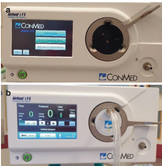
Fig 3 (a) Airseal iFS without Triple lumen filtered tube, (b) Airseal iFS with Triple lumen filtered tube
