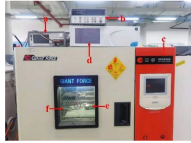
Fig. 9. Experiment platform. a. DC power; b. Logic analyzer; c. Thermostatic controller; d. Pressure controller; e. Acquisition board; f. Resonant pressure sensor.
