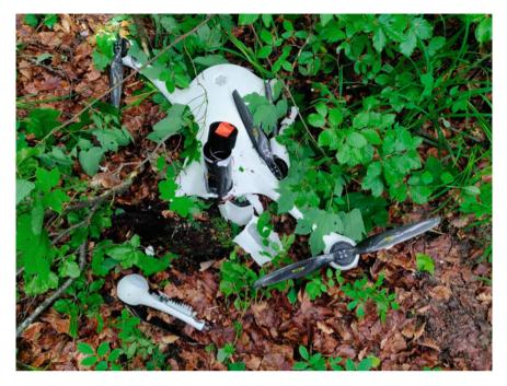
**Fig. 16.1** Matternet (2021) drone which crashed in a wooded area of Switzerland near a kindergarten. The emergency parachute had been deployed, but the chord connecting it to the drone was cut allowing the 12 kg drone to freefall to the ground. Image used with permission, from SUST (2019)
