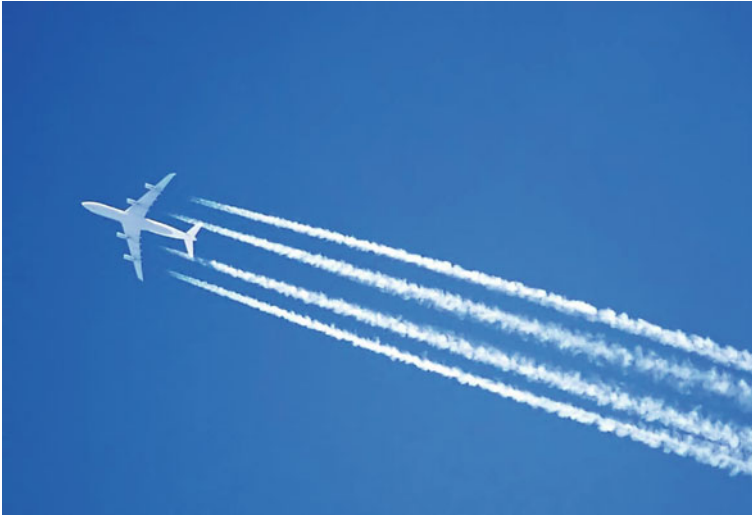
Fig. 8.4 High altitude contrails from a A340 commercial jet airliner (Photo: Adrian Pingstone; curid = 1856927, http://commons.wikimedia.org/wiki/User:Arpingstone )
