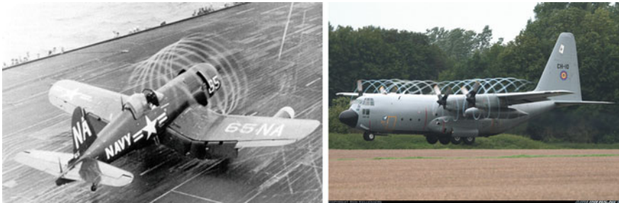
Fig. 8.3 Two examples of tip vortices made visible by atmospheric conditions. At standstill the helix is tight and expands in forward flight as shown at right (Photo at right Belgian Air Force C-130H by Ron Kellenaers # 1131694, Airliners.net)
