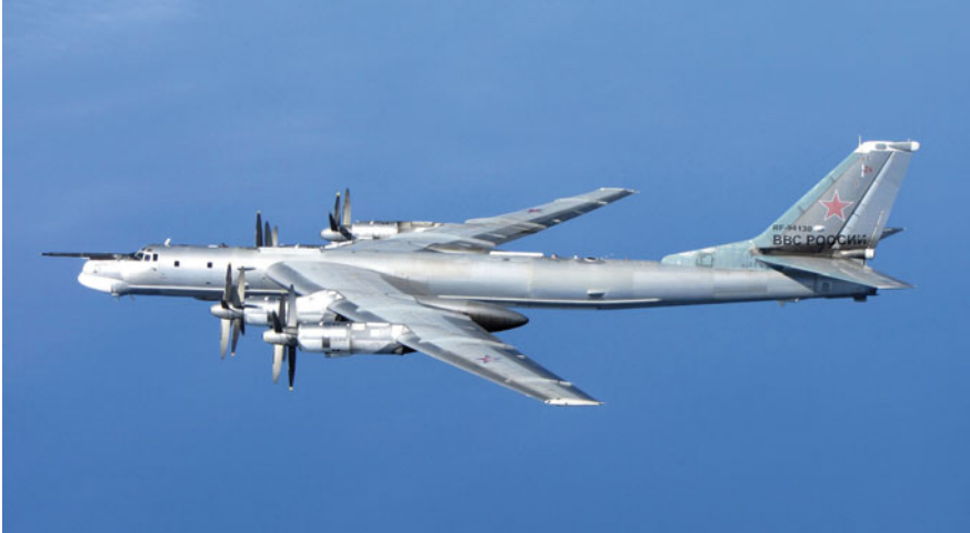
Fig. 8.6 The Cold War Soviet Tupolev Tu-95 strategic bomber using counter-rotating propellers
