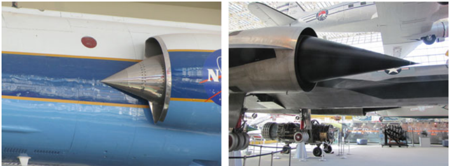
Fig. 13.7 Axisymmetric inlets for supersonic aircraft, F-104 and SR-71. In the lower right background of the SR-71 is a display of a P&W R4360 with its 28 cylinders (Photos taken by the author at the Museum of Flight in Seattle)
