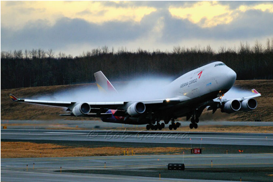
Fig. 5.1 A Boeing 747 at takeoff on a humid day with condensation cloud above the wing (Photo courtesy Bob Garrard)
