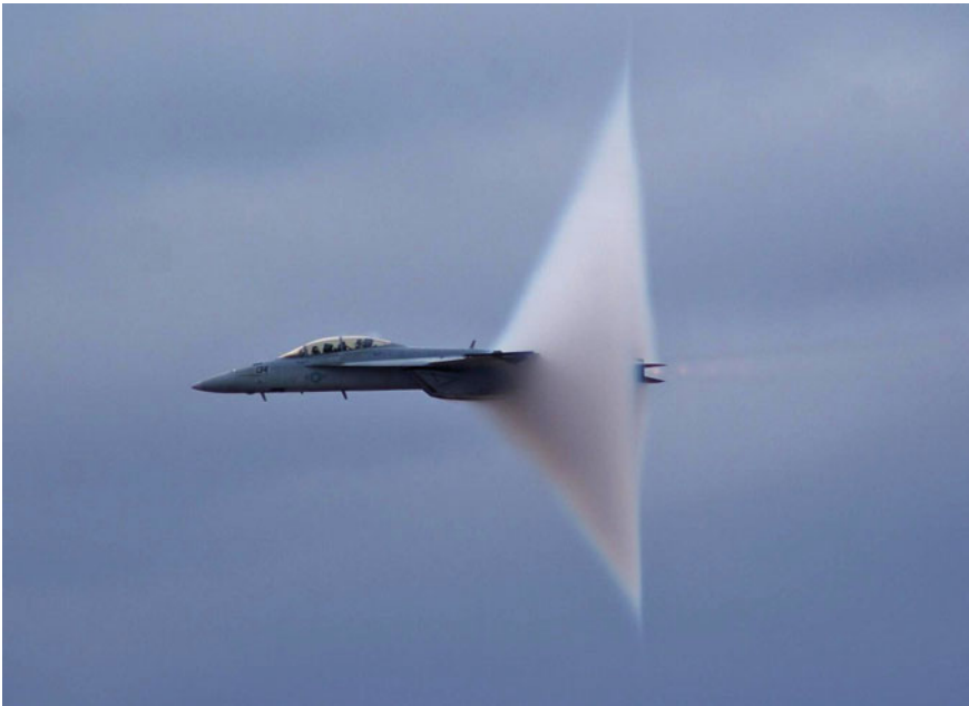
Fig. 7.9 Photo of a F/A-18 in transonic flight in saturated air. The text outlines the argument that the cloud boundary is not a representation of the invisible shock wave system (Photo credit: https://commons.wikimedia.org/w/index.php?curid=15250934 )
