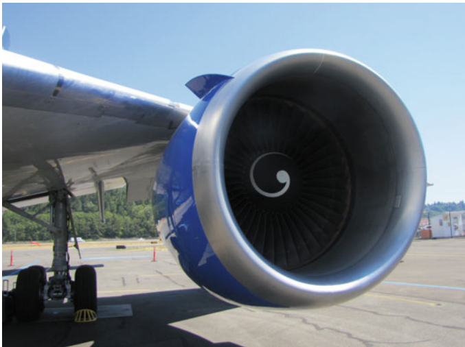
Fig. 13.3 The inlet of a DC-10 airliner wing mounted engine nacelle. One of the two “rabbit ear” vortex generators is located at the 11 o’clock position of the cowling
