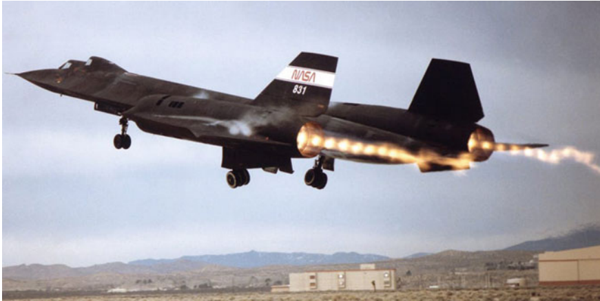
Fig. 13.15 Over- and under-expansion waves in an afterburning J58 propelling an SR-71 (NASA)
