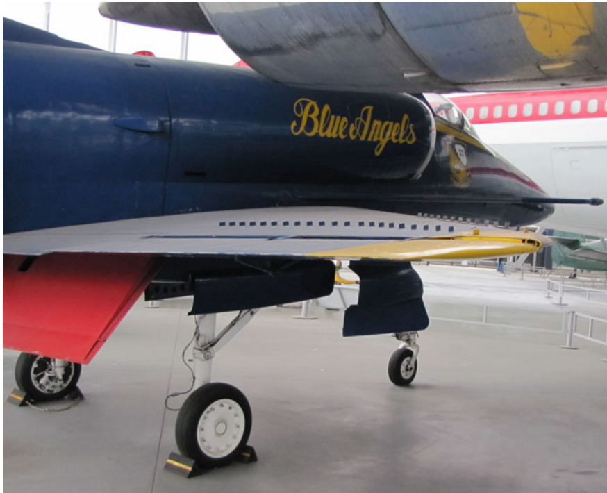
Fig. 4.9 An example of two arrays of VGs on the wing of a Douglas A4D US Navy jet fighter. Museum of Flight display
