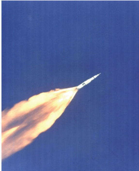
Fig. 13.14 The Saturn V rocket in flight carrying Apollo 11. Note the very large width of the jet from an under-expanded nozzle (NASA)
