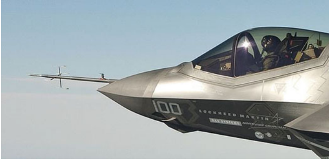
Fig. 6.9 Pitot tube on a Lockheed Martin F-35. This is typically a temporary installation for flight test purposes. This rig measures a number of aerodynamic and attitude parameters. The static measurement is made along the long probe even when flight speed is supersonic [Photo: Wikimedia Commons File:CF-1 flight test.jpg (cropped)]
