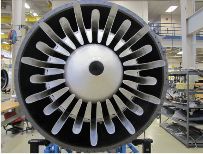
Fig. 13.8 An internal mixer for engine core flow emanating from “behind” the round central cone with the fan flow originating in the surrounding darker space (Photo by author at the service education facility of General Electric in Evendale, Ohio)
