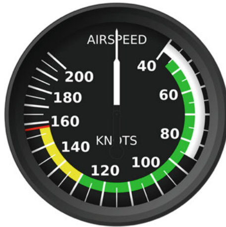
Fig. 6.10 Simple display in an airplane instrument panel showing indicated air speed. In the U.S., this speed is traditionally given in knots (nautical miles per hour). The green zone is safe operation range, yellow requires smooth air, and red tab is the not-to-exceed speed for concerns of structural damage to the airplane. The white range is for operation with flaps, such as during takeoff or landing. More complex versions of such a dial are common (Wikimedia Commons: Marek Cel, file: Airspeed indicator.svg)
