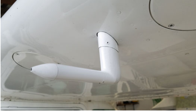
Fig. 6.8 Pitot probe under the leading edge of a Cessna 172. The ports for measuring static pressure are on the airplane fuselage (Photo: Ronald Parker)
