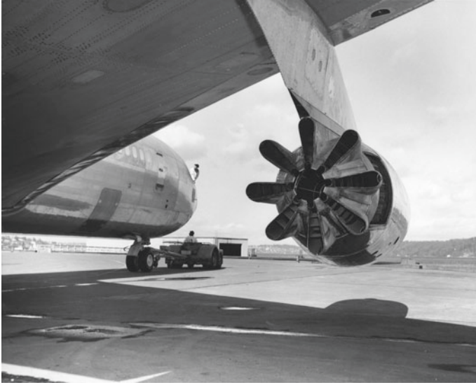
Fig. 13.9 An early turbofan engine on a Boeing 707 (a Rolls-Royce Conway) with a daisy petal mixer that joins the external and the primary core flow of the engine. In this engine, the fan flow exits through two nozzles on the sides of the nacelle. These nozzles are partially obscured in this view but the visible one exits the nacelle between 2 and 4 o'clock positions (The Boeing Company)
