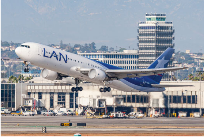
Fig. 13.4 A LAN (Argentina) Boeing 767 taking off from Los Angeles. The white “cloud” just inside the inlet is water vapor condensation at the minimum flow area where static temperatures are lowest and, in this case, below the dew point (Photo courtesy Werner Horvath, Airlines.net)
