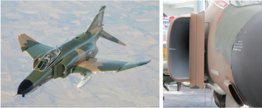
Fig. 13.5 A McDonnell F-4 in flight showing the shock generation ramp on the inlet and the boundary layer diverter between the inlet and the fuselage (Picture credit: USAF—holloman.af.mil, curid = 50920146 ). At right is the Museum of Flight display showing the diverter head-on. Note the small diverter on the scoop at lower right and the inlet instrument probe
