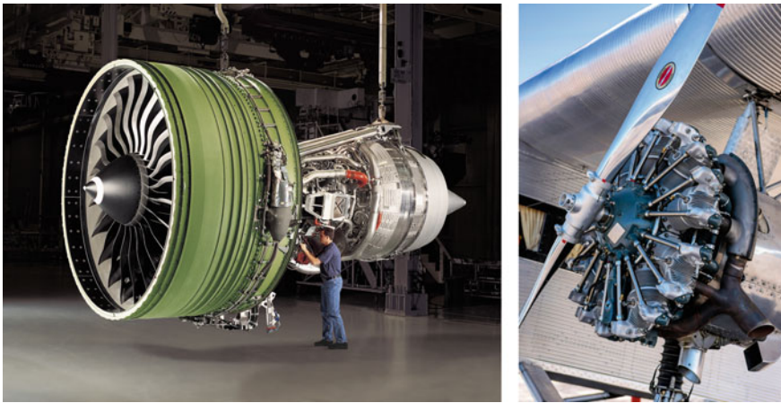
Fig. 11.2 A modern turbofan engine: GE90-115 (mid 1990s) contrasted to a radial Wright 9-cylinder Whirlwind on a Ford Trimotor (1929); not to the same scale (Courtesy General Electric and agefotostock; Christopher L. Smith)
