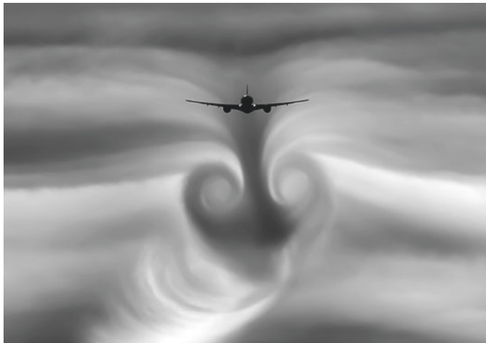
Fig. 2.3 An airplane flying through a cloud layer displaying the downwash and the associated and necessary wing tip vortices (Credit: istock.com: image 1125702712/alextoV)
