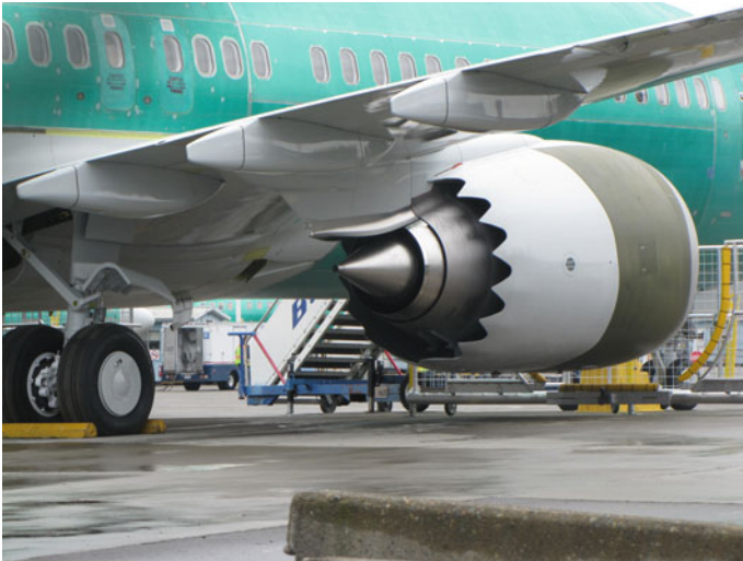
Fig. 13.10 The (convergent and scalloped) fan flow nozzle exit lip of a commercial airliner, a Boeing 737 MAX. Both core flow and fan flows are partially expanded against the conical, external nozzles (Photo by author at the Boeing assembly plant in Renton, Washington)
