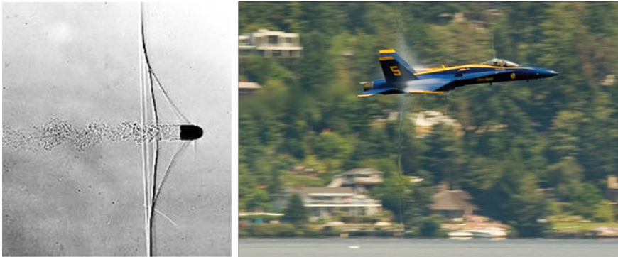
Fig. 7.5 Left: A shadowgraph of a bullet in supersonic flight. Weak oblique waves from the nose coalesce into an oblique shock that turns into a normal shock further out. Note the turbulence in the wake (Photo: Daniel P.B. Smith, Creative Commons, 1962; https://en.wikipedia.org/wiki/Doc_Edgeron#/media/File:Shockwave.jpg ). Right: Shock image generated by a low-level fly-by of a US Navy “Blue Angels” F/A-18. Note the wing recompression shock above and below the wing trailing edges (above and below the number “5”) as well as shocks at the leading edge and above the cockpit. Its visibility is due to the refraction from the air density change across the shock. There is also a faint amount of condensation above the low-pressure, upper side of the wing (Image courtesy Barry Latter)
