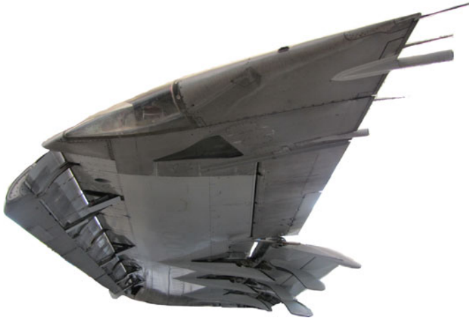
Fig. 2.2 A wing of a Boeing 727 with all high lift devices deployed (Photo by author, Museum of Flight, Seattle)
