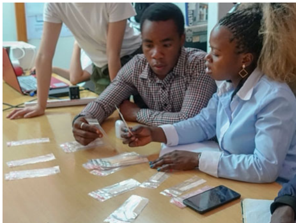
Fig. 9.6 Counting the colony number of total coliforms by the workshop participants. (Photo by Kataoka)
