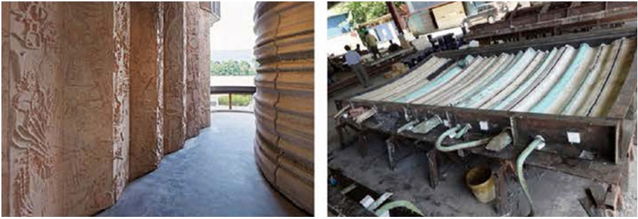
Fig. 8. Adjustable silicone moulds in NTU ([Adjustable silicone moulds] n.d. [image online] Available at: < http://www.designcurial.com/news/dim-sum-towers-heatherwick-studios-learning-hub-in-singapore-4593669/4 > [Accessed 16 June 2018].)
