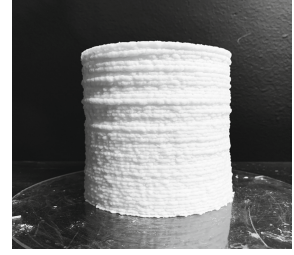
Fig. 27. Decline angle limitation testing: The decline angle limitation testing shows that, while the material is in wet state, the angle limitation is around 20 degree. But once we blow it with hot wind to speed up the water evaporation, the angle limitation is significantly improved.
