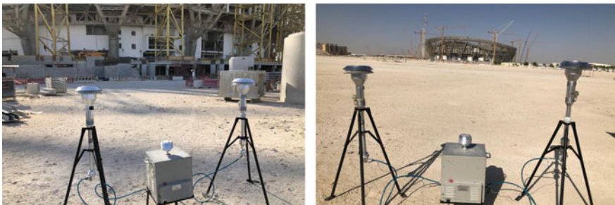
Fig. 7.6 Dust testing around the stadium
