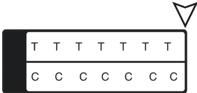
Fig. 51.3 Tensile and compressive force mechanism
