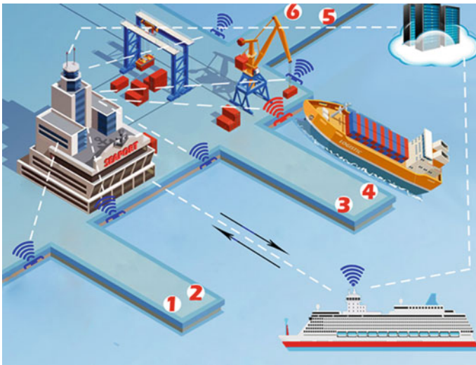
Fig. 2 High-level design of the smart berthing system for ships
