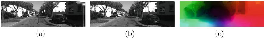
Fig. 2. Two subsequent frames from Seq 00 and corresponding dense optical flow. (a) and (b) show the raw images and (c) shows the dense optical flow (Color figure online).
