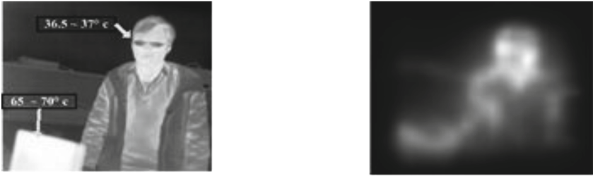
Fig. 2. An example of an Infrared Thermal Image (a) and its saliency map of (b).
