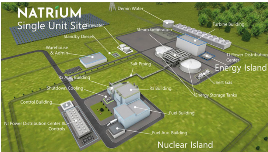
Fig. 6.15 Natrium single unit site layout. Source TerraPower LLC
