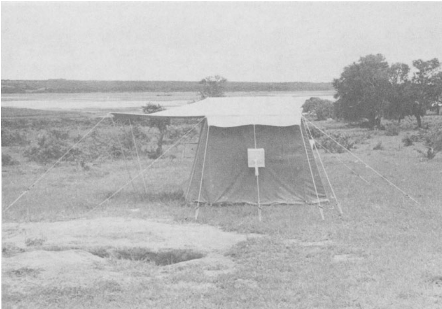
FIG. 5.6. A side view of an experimental tent showing three of the four window traps and the roof overhang covering the entry slits (photograph courtesy of B. Sharp).
