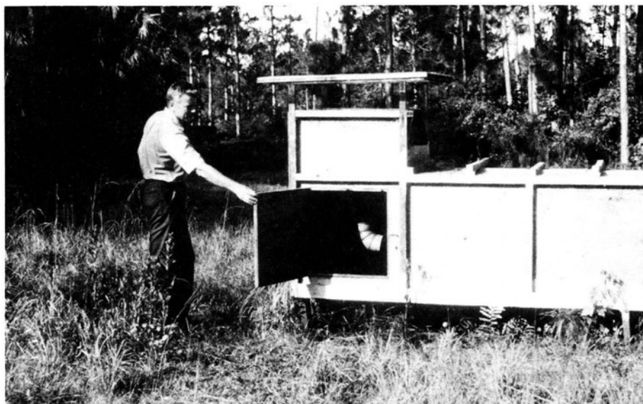
FIG. 4.14. Example of a typical L-shaped suction trap of Bidlingmayer (1974) (M. W. Service).
