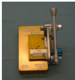
Fig. 1. Cutter designed to cut Personna single-edge prep blades
