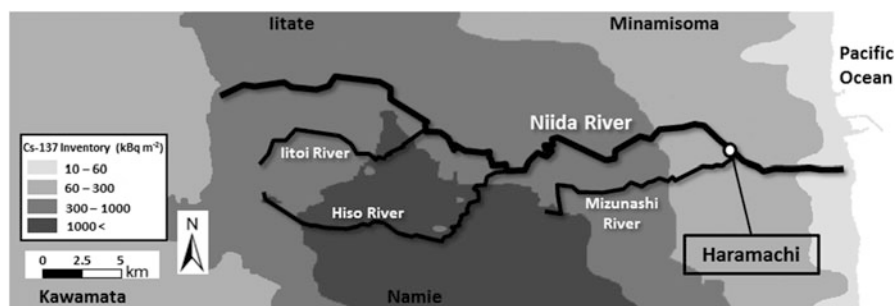
Fig. 6.1 Map showing the sampling site (Haramachi) located 5.5 km upstream from the Niida river mouth along with the spatial ^{137}\text{Cs} inventory from MEXT [6]. Total SS was collected continuously from December 2012 to January 2014 using a time-integrative SS sampler
